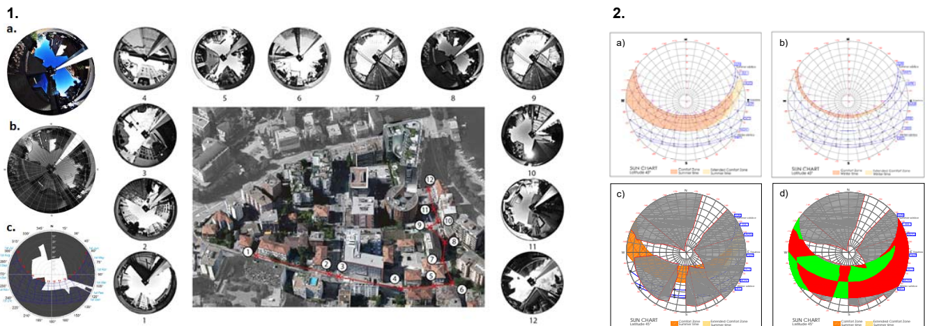
Figure 3: Simulation tools and photographic diagnosis analysis: 1) Sky-factor assessment through photographic method, different steps in the image processing: (a) Image modification in HDR format; (b) Image for the actual situation; (c) and software simulation for a possible design scenario; 2) Comfort zone calculated and represented in the solar polar sun-path diagram (stereographic projection) for Lugano area. Source: Polo López C. S. ISAAC-SUPSI [2]
